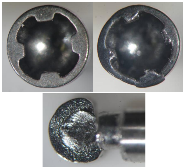
Figure 9. Interior details of the BHS driver coated with DHC without testing (left), after testing (right) and breakage surface of the upper part of the driver (bottom).
