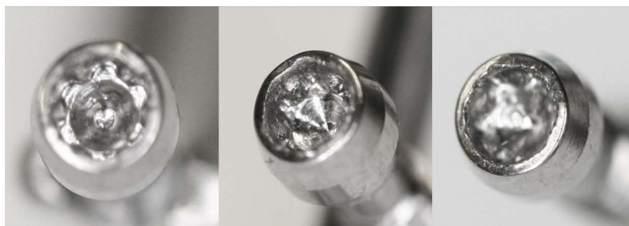
Figure 14. Original Hexalobular screw (left) and tested screws (centre and right).
