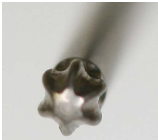
Figure 13. Hexalobular driver after testing (right).
